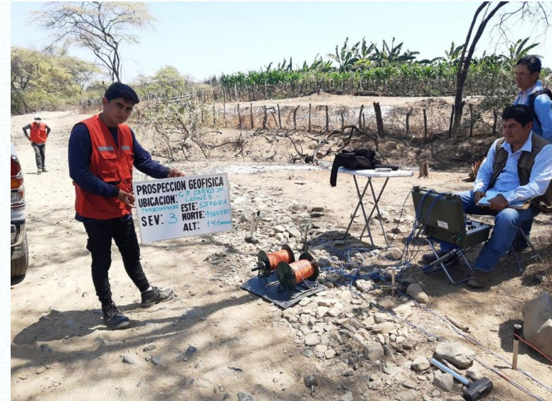
Hired Sub-Consultant (Remicio Y Gutierrez) Performing Hydrogeologic Evaluation in Las Mercedes KM11 to Determine Groundwater Availability. (2022-09-15)
